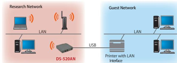
This example shows the use of the DS-520AN as a wireless resource. The DS-520AN can also be used as a second LAN interface (wired). It is not possible to simultaneously use it as a WLAN and LAN print server.
