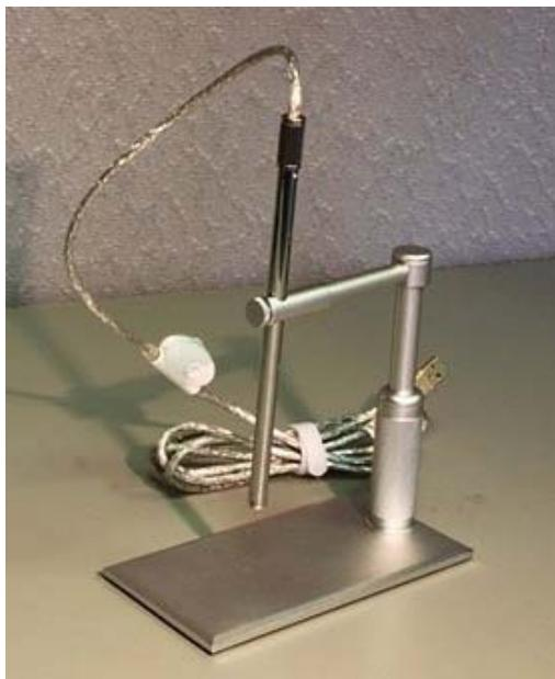
The tubular imaging system consists of an optical lens and image sensor, an illumination mechanism and an image transfer control circuit which connects to your computer via the USB port.
